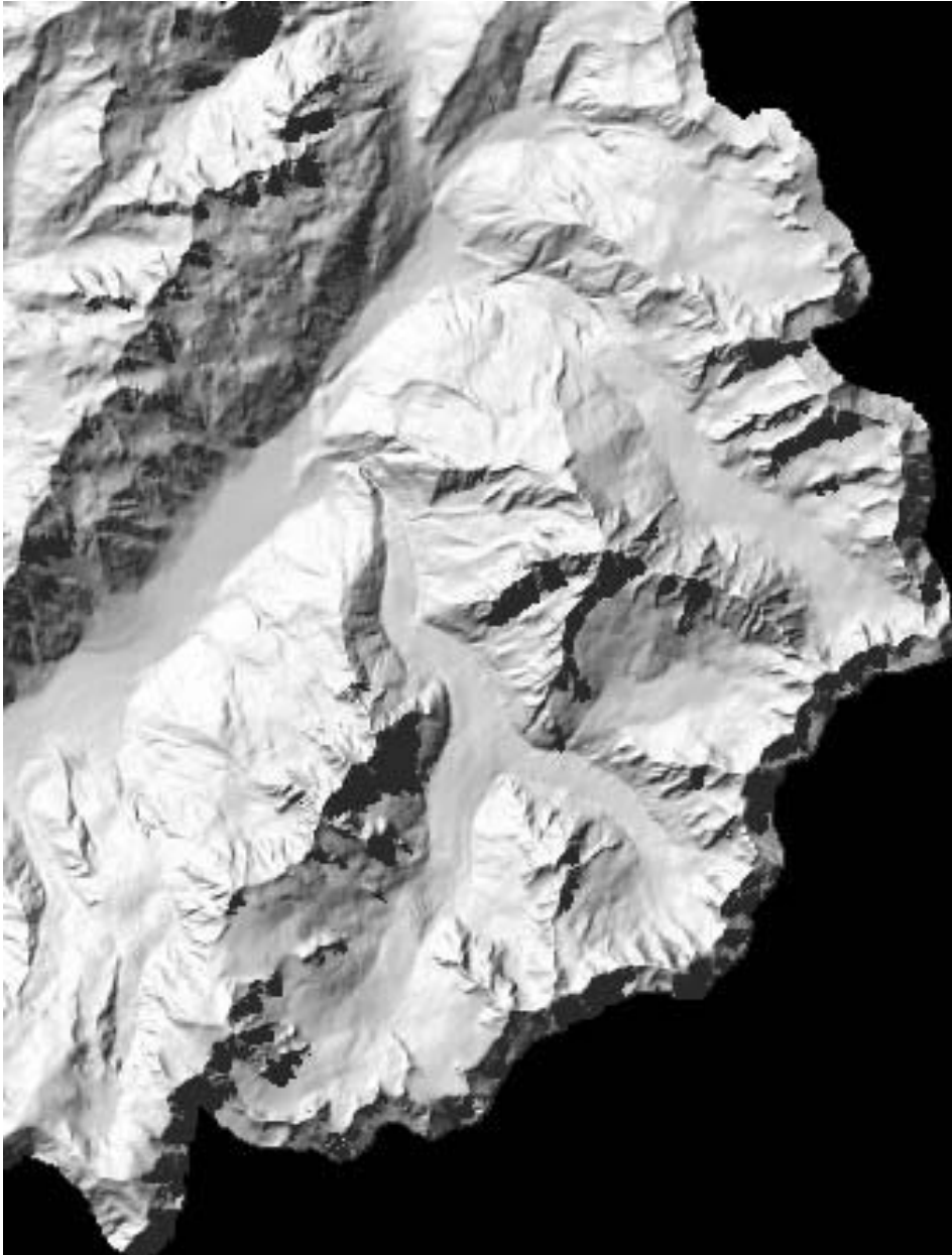
Figure 7. Hillshading of Mont Blanc DEM. The incident light is modified according to the cosine angle of incidence of the Sun on the slope. A minimum illuminance of 18% is introduced to account for diffuse radiation. Illumination is from the North-west at 45^\circ elevation.
