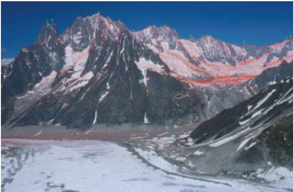
Figure 5. Superimposition of the perspective projection of a DEM of the Mer de Glace (figure 4) over a photograph of the area. Red dots are the perspective projections of the original DEM grid cells, and green dots are the ground control points (GCPs). The GCPs are located on prominent points, such as the peaks on the ridge, and should be easy to identify on the image for fast photograph orientation. The photograph is taken from the Refuge du Requin looking east-north-east.
