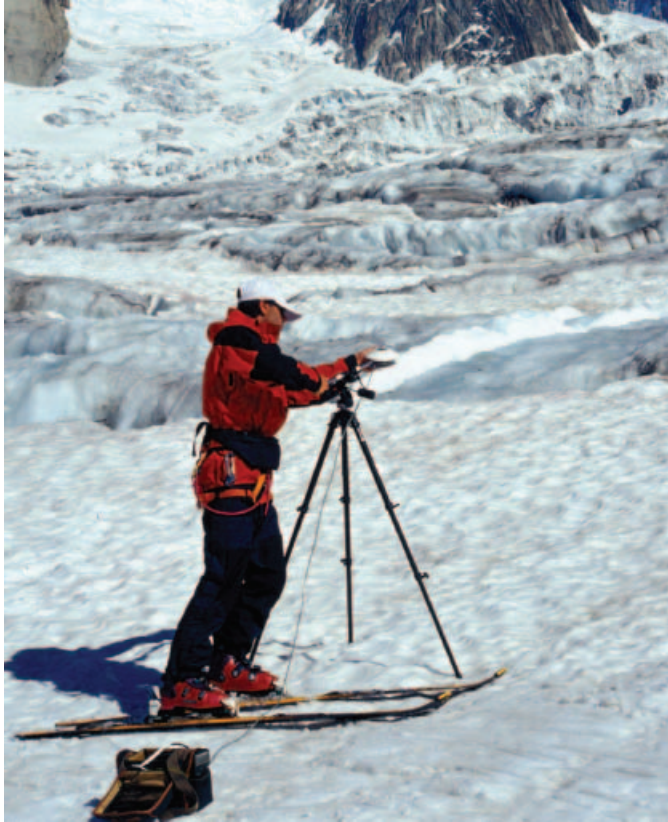
Figure 12. Albedometer setting. The white oval, above and right of the camera tripod, is the albedometer, made up of two Kipp & Zonen opposed pyranometers. The output is read in two voltmeters connected at the extreme of the cable in the bag below the skier-operator in the image.
